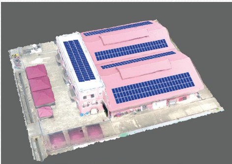
Optimum PV system layout for maximising solar energy generation throughout the year, including shading analysis
