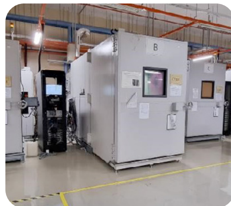
Large-volume climate chamber for reliability testing
