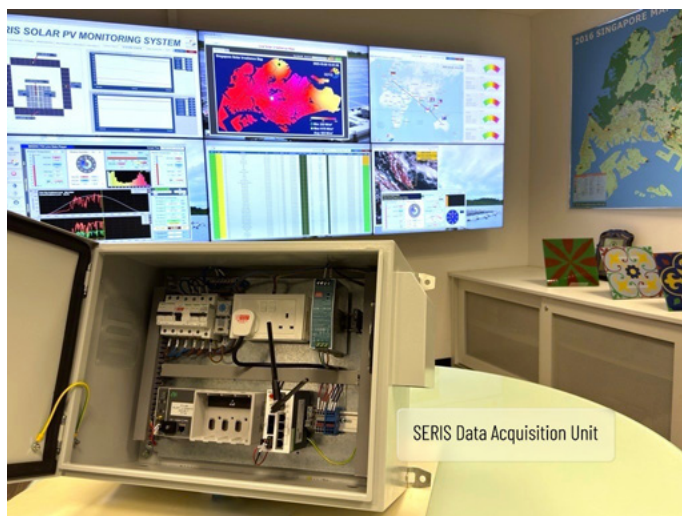
SERIS remote data acquisition station for PV Asset management
