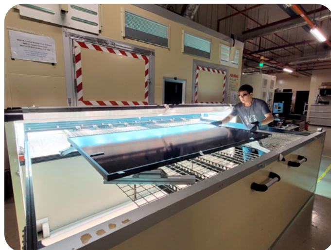
Fig. 1: UV chamber at SERIS' ISO/IEC 17025-certified PV module testing laboratory for quantifying the impact of UV-induced degradation (UVID)
