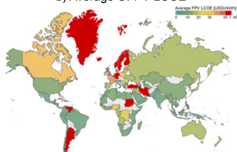
Fig. 2: Global potential of offshore FPV systems: a) offshore area required to fulfil the region's electricity demand; b) average LCOE from OFPV in water spaces considered in a)
