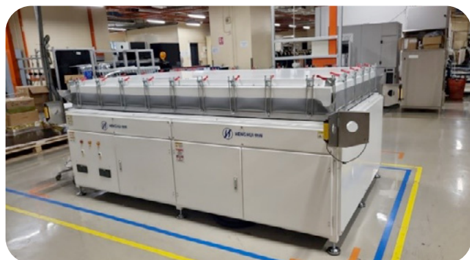
Semi-automatic PV module laminator (HengHui HB-C6D)
