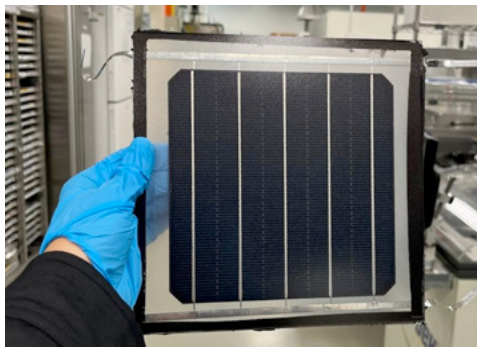
Fig. 4: Photograph of a fully in-house fabricated 244-cm 2 (M2-size) perovskite-silicon 1-cell tandem mini-module featuring low-temperature encapsulation and interconnections.
