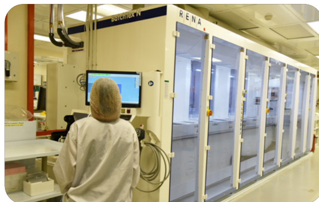
Inline wet-chemical processes (both acid and alkaline chemistries) for silicon wafers, including cleaning and etching
