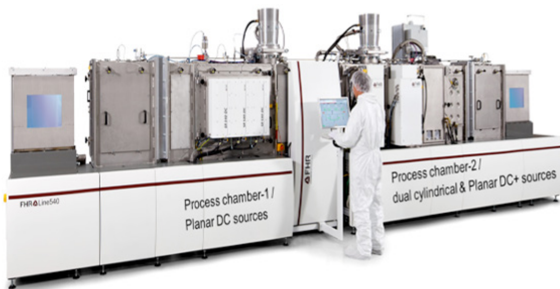
In-line multi-chamber magnetron sputtering machine at SERIS
