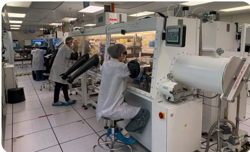
Several compartmental gloveboxes in the Perovskite Laboratory dedicated to various processes such as synthesis, deposition, metallisation and characterisation of perovskite materials and solar cells
