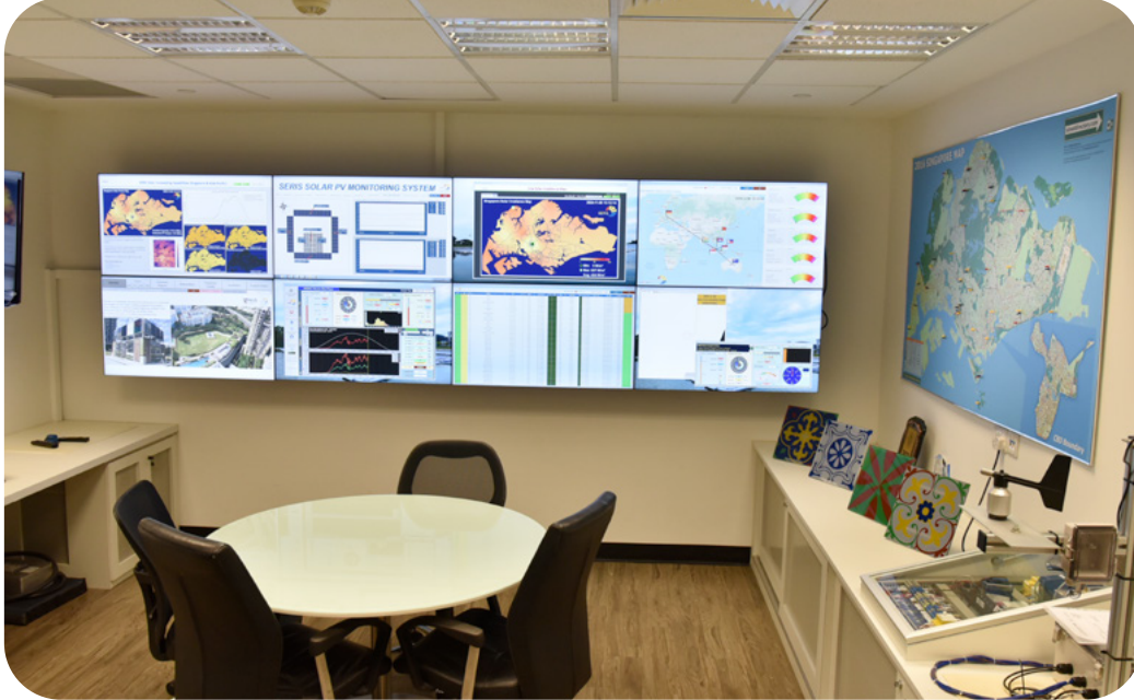
The PV System Monitoring Lab's video wall, displaying the live solar irradiance map of Singapore (also available at www.solar-repository.sg/solar-irradiance-map ), real-time performance data of several rooftop PV systems, as well as real-time meteorological parameters from several remote stations deployed across Singapore
