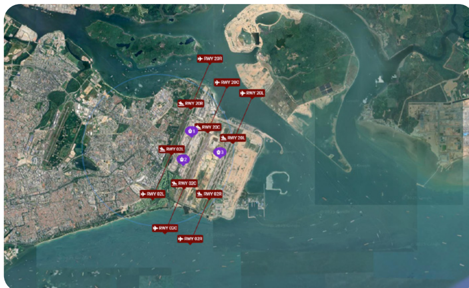
A typical setup for a glare analysis project: ATCTs and flight paths considered for glare analysis for a PV installation within Changi Airport, Singapore
