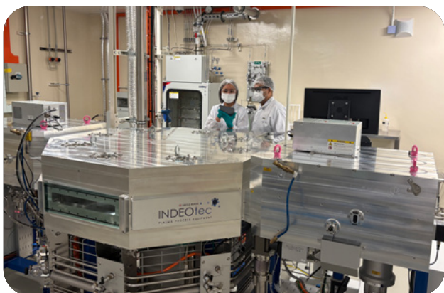
PECVD tool for deposition of intrinsic and doped amorphous silicon layers for heterojunction silicon wafer solar cells
