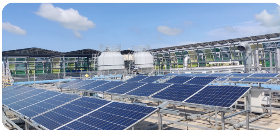
SERIS' Outdoor Module PID Test Facility
