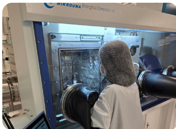
Glovebox-integrated thermal evaporator for thin film deposition of metals and inorganic and organic functional layers
