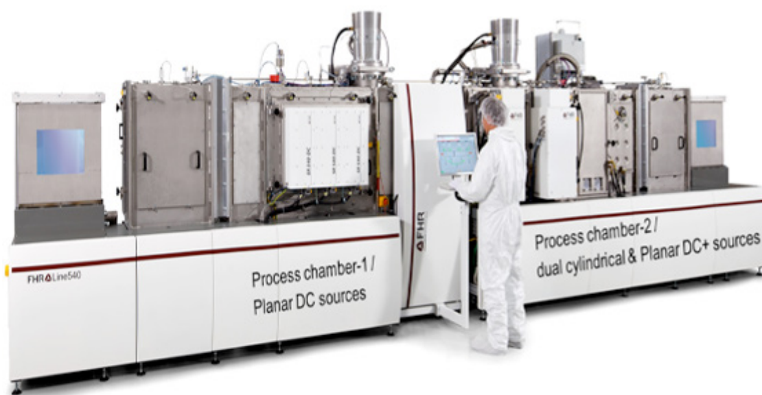
In-line multi-chamber magnetron sputtering machine at SERIS
