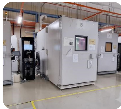
Large-volume climate chamber for reliability testing
