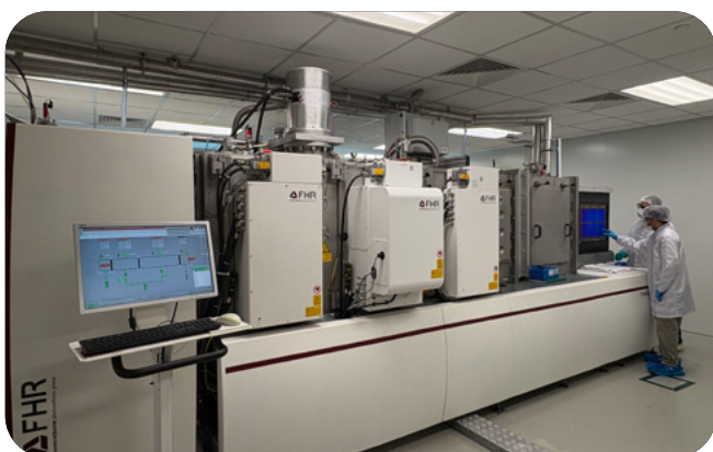
PVD sputtering platform for depositing metal layers, transparent conductive oxides and multi-layer stacks on silicon wafer solar cells and perovskite thin-film solar cells
