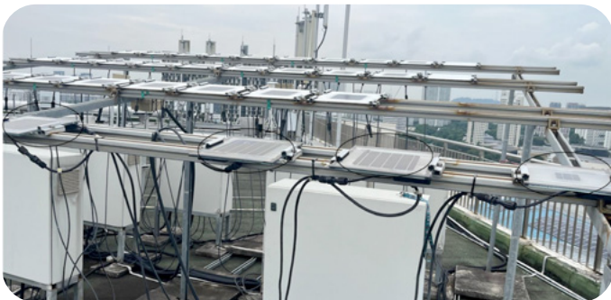
Fig. 7: Perovskite-silicon tandem mini-modules deployed at the NUS Rooftop Testbed for outdoor testing in Singapore's hot-humid tropical climate.
