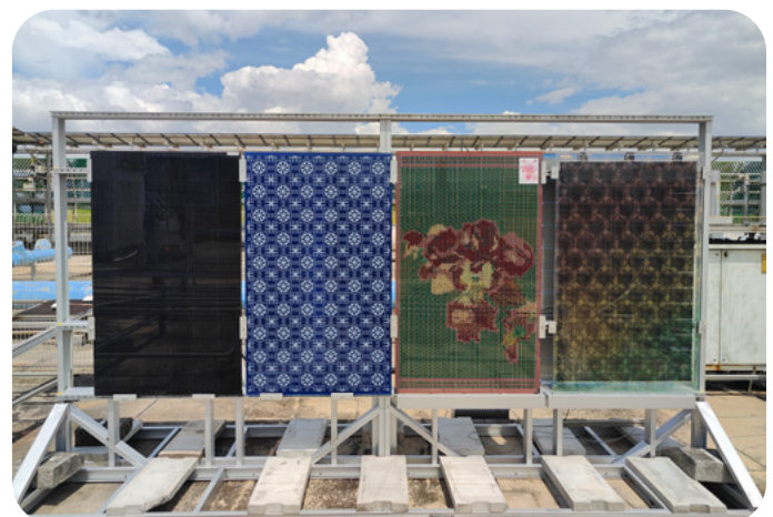
Fig. 3: BIPV outdoor testbed at the Cleantech One rooftop. The testbed will be used to evaluate various technologies as well as mounting and interconnection strategies.
