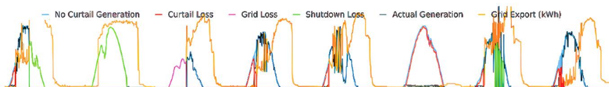
Figure 3: SGR reconstructing a PV system's profile as if it generated normally without curtailment loss, shutdown loss and grid loss; revealing 21.2% curtailment loss, 22.2% shutdown loss and 4.0% grid loss from selected period which previously were hidden as low system performance.
