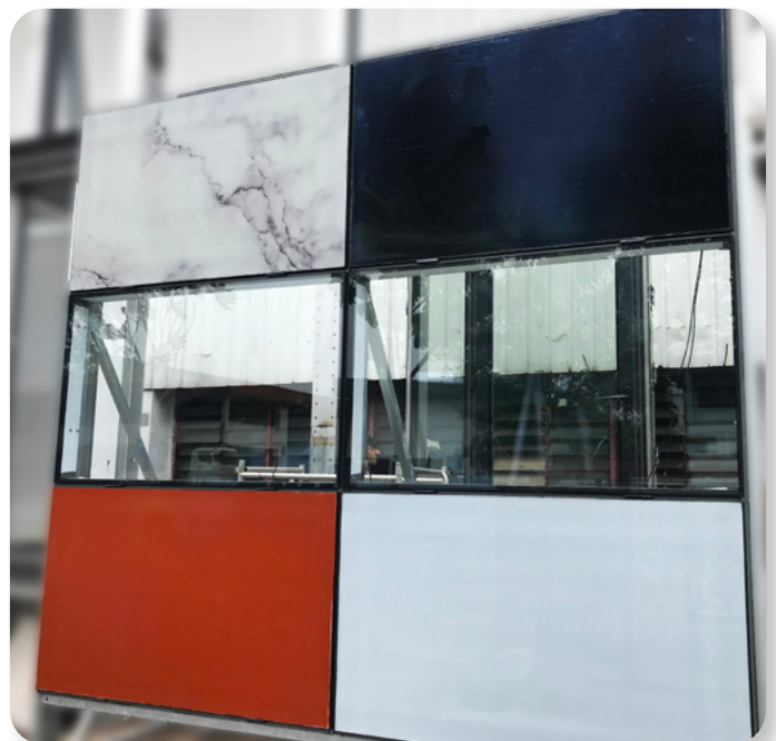
Fig. 2: Coloured BIPV modules that mimic building materials, seamlessly integrating into the built environment
