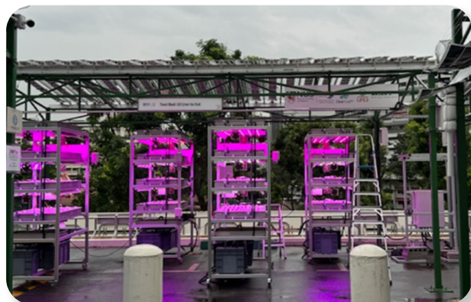
Fig. 3: SERIS' testbed 2 in the Yuhua Agritech Solar (YAS) Living Lab with a hydroponics system consisting of horizontally layered growing beds.
