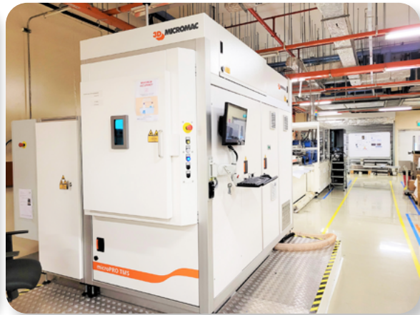
Automatic solar cell stringer (left) and TLS solar cell cutter (right) in SERIS' PV Module Development Laboratory located at CleanTech Park
