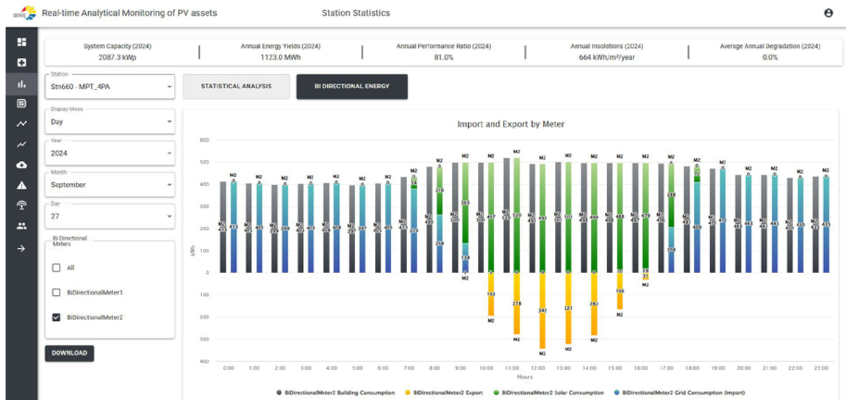
Fig. 4: Screenshot of the SERIS Energy Management platform, showing energy export during the day (yellow bars with negative values)
