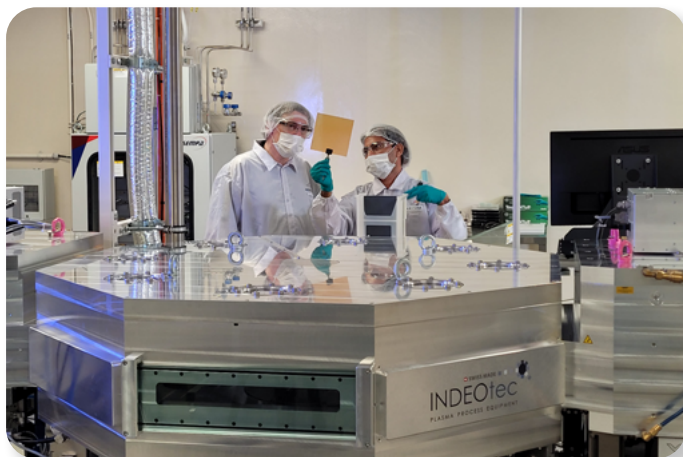
PECVD tool for deposition of intrinsic and doped amorphous silicon layers for applications in heterojunction solar cells.
