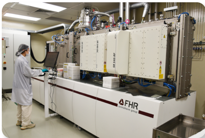
The PVD sputtering platform at SERIS is used for depositing metal layers, transparent conductive oxides and multi-layer stacks for silicon and thin-film solar cells, as well as heterojunction silicon wafer solar cells.
