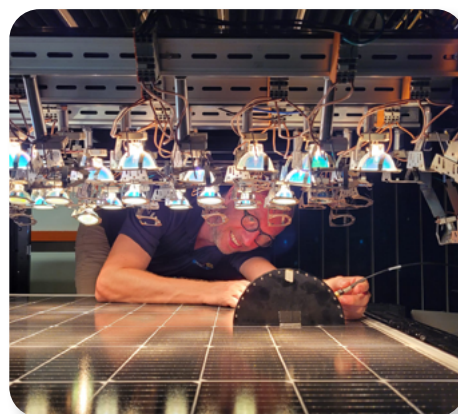
Measurement of the IAM of a commercial-size PV module
