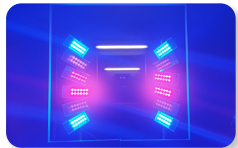
Complementary coloured light bias system in one of SERIS' Class A+A+A+ solar simulators
