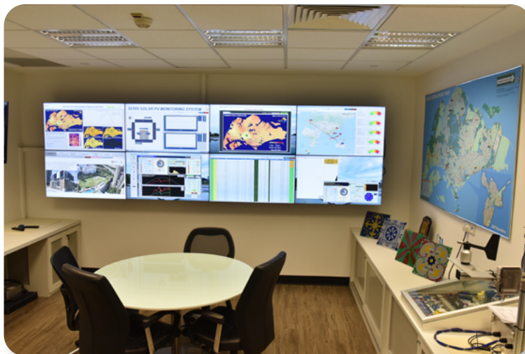
The PV System Monitoring Lab's video wall, displaying the live solar irradiance map of Singapore (also available at www.solar-repository.sg ), real-time performance data of several rooftop PV systems, as well as real-time meteorological parameters from several remote stations deployed across Singapore.
