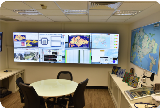
PV Monitoring Display Panel with live display of irradiance, sky images, and weather parameters
