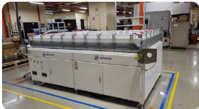
Semi-automatic PV module laminator (HengHui HB-C6D)
