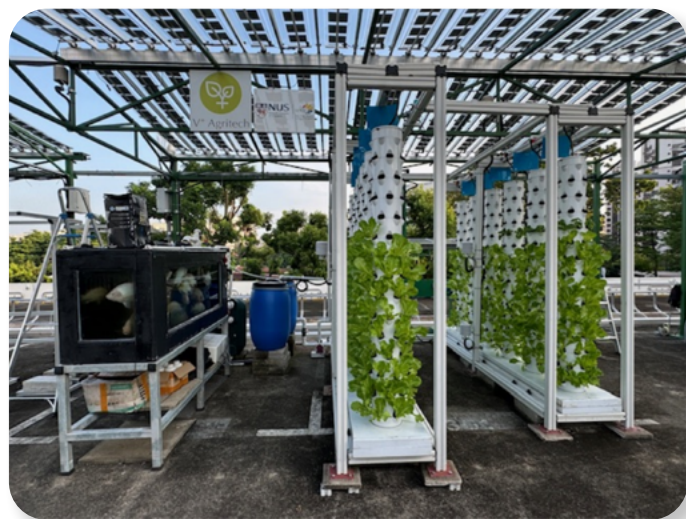
Fig. 2: SERIS' testbed 1 in the Yuhua Agritech Solar (YAS) Living Lab with an aquaponics system consisting of vertical growing towers.
