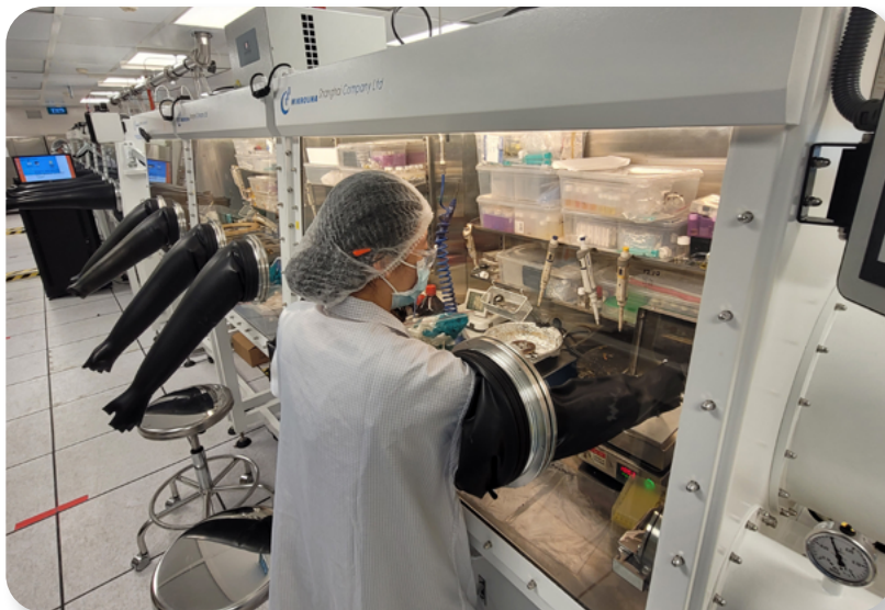
Several compartmental gloveboxes in the Perovskite Laboratory dedicated to various processes such as synthesis, deposition, metallisation and characterisation of perovskite materials and solar cells.
