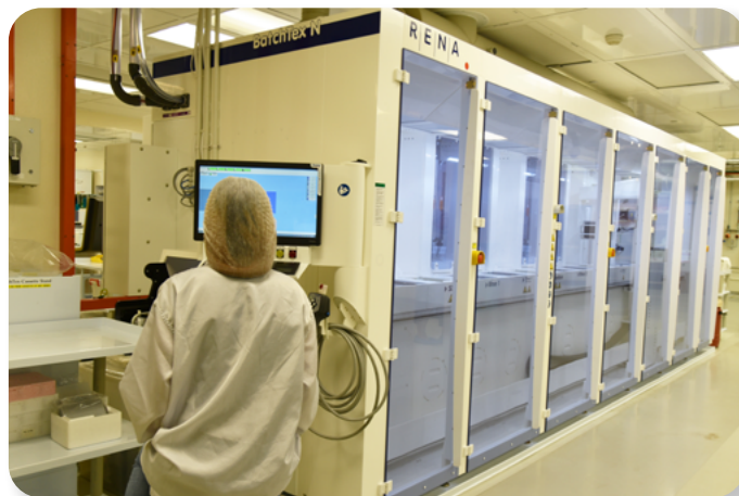
Inline wet-chemical processes (both acid and alkaline chemistries) including cleaning and etching.
