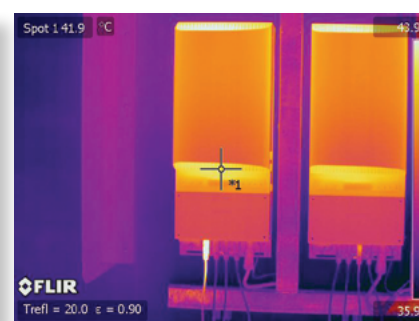
Thermographic analysis showing the overheating of a DC cable and a connector
