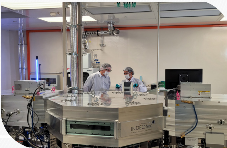
PECVD tool for deposition of intrinsic and doped amorphous silicon layers for applications in heterojunction solar cells.
