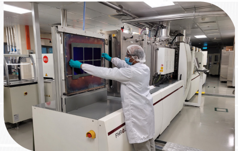
The PVD sputtering platform at SERIS is used for depositing metal layers, transparent conductive oxides and multi-layer stacks for silicon and thin-film solar cells, as well as heterojunction silicon wafer solar cells.
