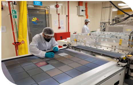
A unique prototype PECVD tool for ultra-fast deposition of doped silicon and metal oxide thin films in SERIS cleanroom
