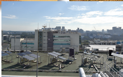
SERIS' Outdoor Module Testing facility in Singapore (tropical climate)
