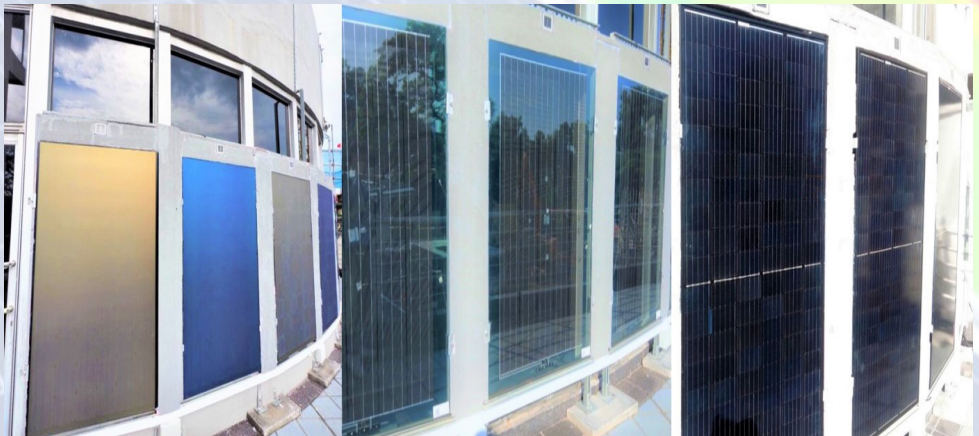
BIPV façades testing of performance and thermal properties at the School of Design and Environment at the NUS Campus
