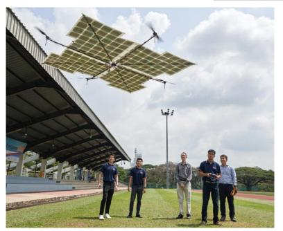
With 148 IBC silicon solar cells, the NUS Solar Helicopter Team announced that 100% solar-power flight had been achieved in a quadcopter! With full controllability (by remote control), under natural sunlight, the aircraft had no battery on board.
