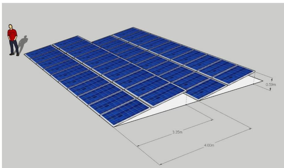
*Figure 5.6: Two-row configuration of a solar array used for deriving the “area factor”. The gap between rows is sufficiently large to avoid row-to-row shading and to enable maintenance access.*
