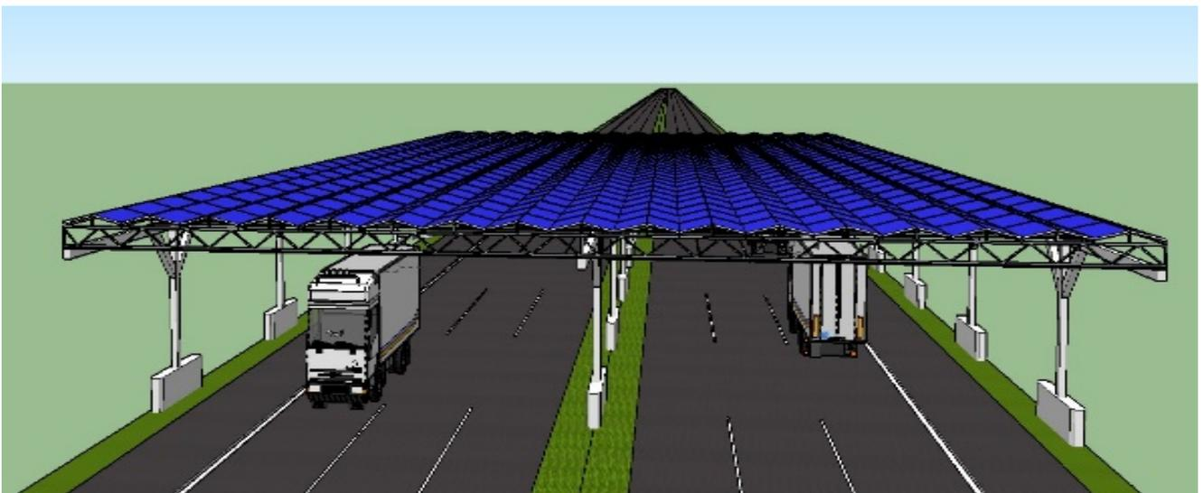
*Figure 5.3: Artist impression of a retractable system over-arching existing roads. Source: iWorks AG.*
