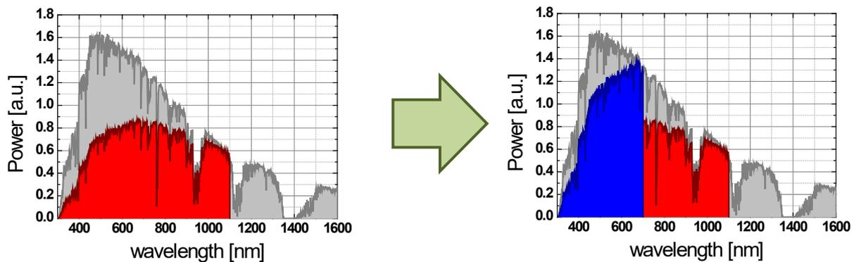
*Figure 5.5: Generic principle of better harvesting the solar spectrum through double junction solar cells (tandems)*
