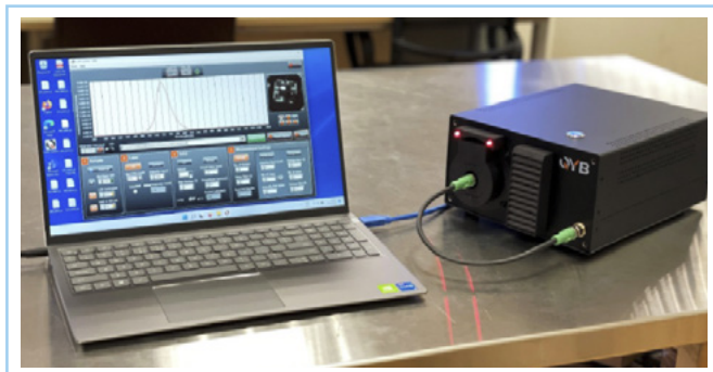
(Top) Photo of upgraded time-resolved fluorescence spectrometer with added micro-luminescence characterisation capabilities. (Bottom) Photo of new characterisation tool for voltage loss analysis of perovskite solar cells, using the photoluminescence quantum yield technique.
