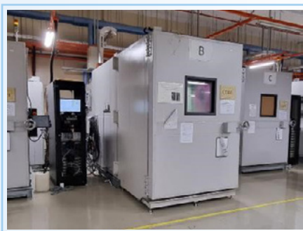
Large volume climate chambers for reliability testing
