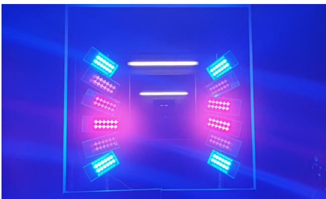
Coloured bias light system and example of EQE measurement on a double-junction amorphous silicon PV module.
