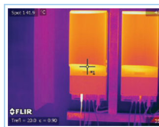
Thermographic analysis showing the overheating of a DC cable and a connector.
