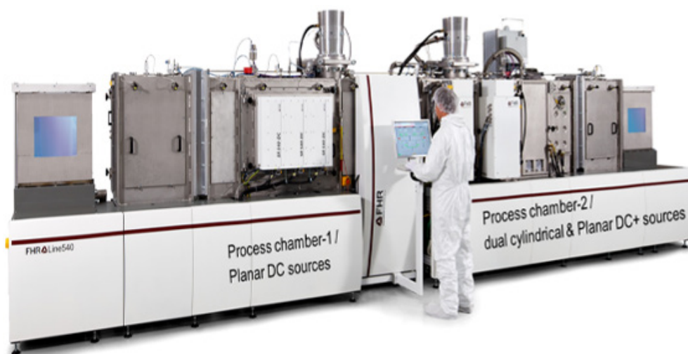
In-line multi-chamber magnetron sputtering machine at SERIS
