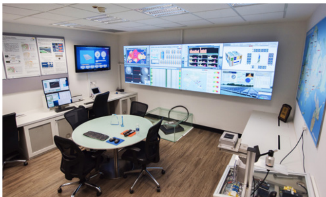
PV Monitoring Display Panel with live display of irradiance, sky images, and weather parameters
