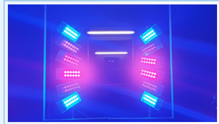
Complimentary coloured light bias system in one of SERIS' Class A+A+A+ solar simulators
