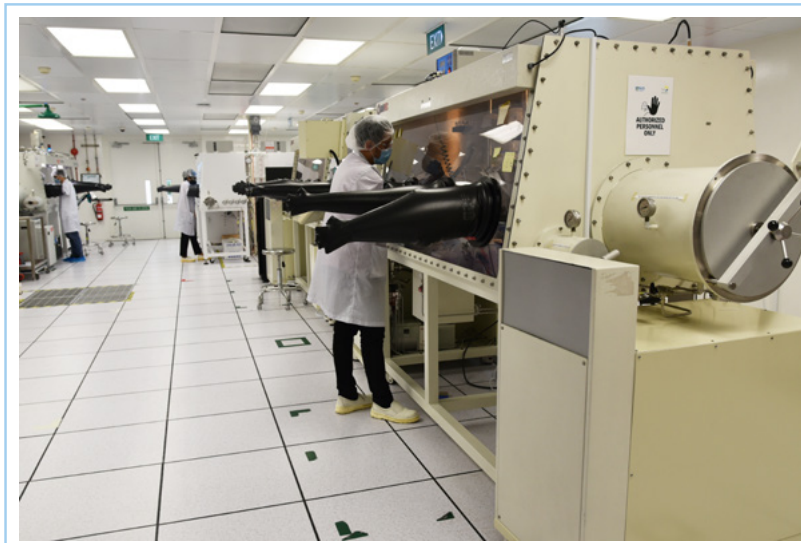
Several compartmental gloveboxes in the Perovskite Laboratory dedicated to various processes such as synthesis, deposition, metallisation and characterisation of perovskite materials and solar cells.
