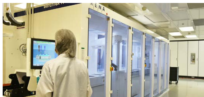
Automated batch tool for wet-chemical processing
