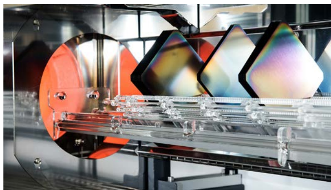
View into the load station of the furnace
