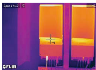
Thermographic analysis showing the overheating of a DC cable and a connector.
