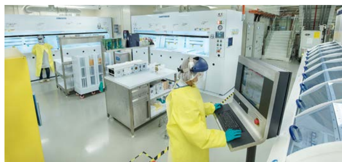
Inline wet-chemistry tool for single-side processing of silicon wafers
